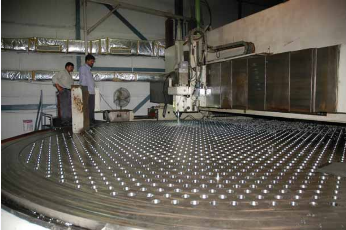
Machining of top plate for Grid Plate.
