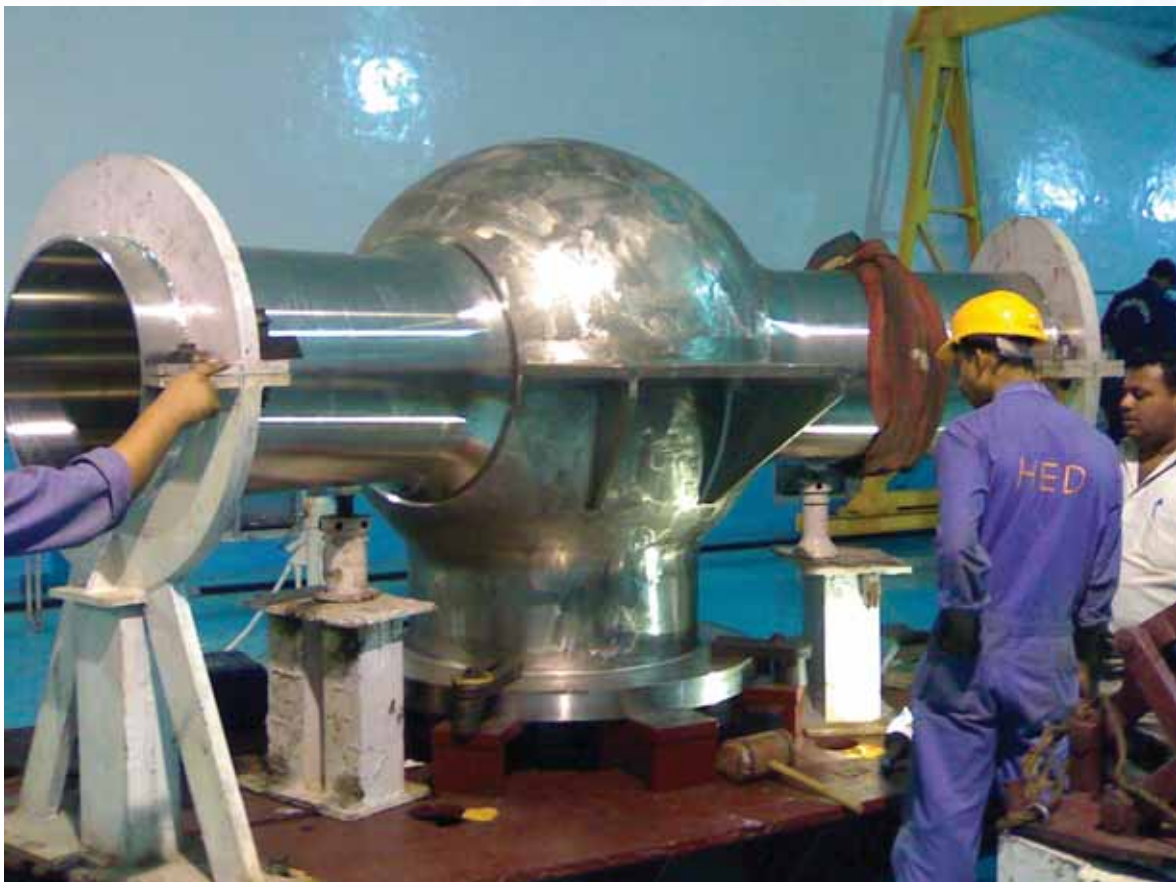
Primary pipe-spherical header with nozzles.
